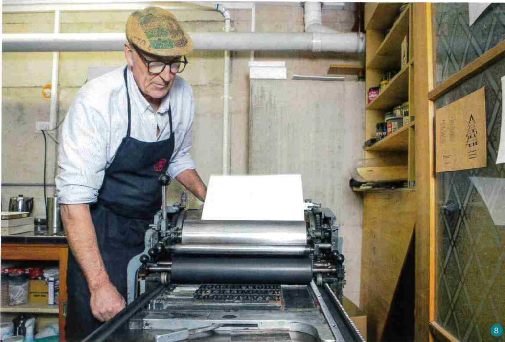
8. Tait-Jamieson proofing Hebrew wood type on a Vandercook press. 9. Trial page of Monotype for a fine edition. 10. Fillet wheels for bookbinding. 11. Linecaster keyboard and matrices.
